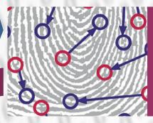
Unique points identified A template is created by the software that shows the intersection of unique points on the finger. The fingerprint image is destroyed. The template is converted to a binary number. The binary number is then encrypted and stored.
